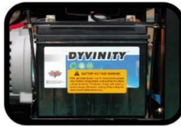
STEP 2. Connect the battery before starting.
