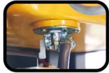
STEP 6. Turn the fuel switch on.
