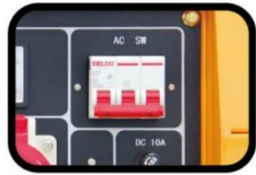
STEP 3. Turn the circuit breaker off.
