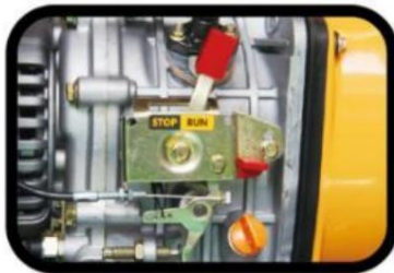
STEP 7. Pull the speed control lever to "RUN" position.
