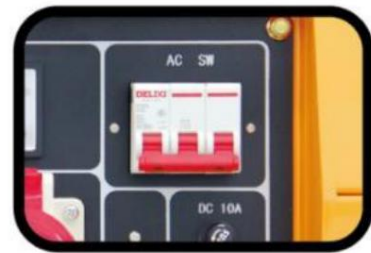
STEP 3. Turn the circuit breaker off.
