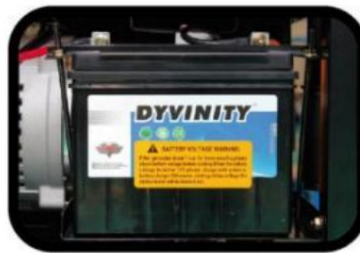
STEP 2. Connect the battery before starting.
