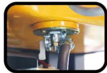
STEP 6. Turn the fuel switch on.
