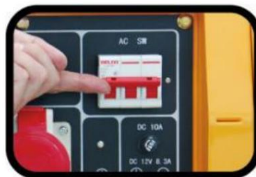
STEP 11. Turn the circuit breaker on.
